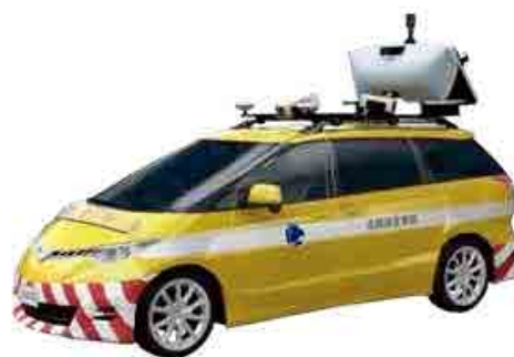
図 4.1.3 MMS (Mobile Mapping System)
