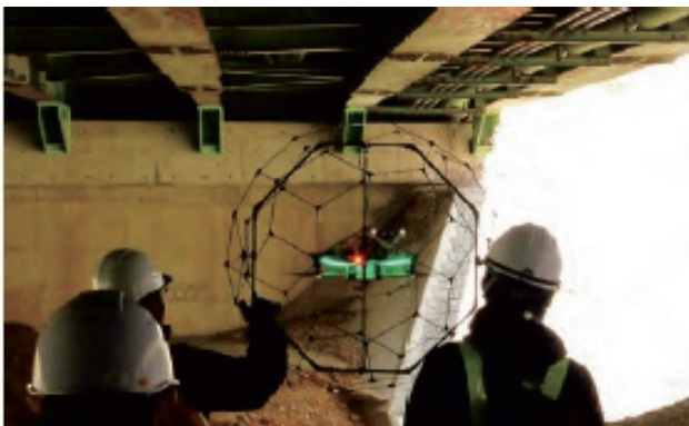
Fig. 2 Demonstration testing of spherical shell drone on bridge substructure
