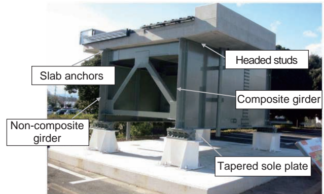
Fig. 5 View of the steel bridge model
