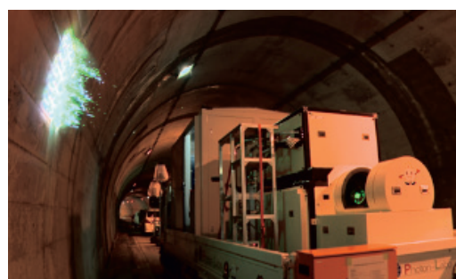
Fig. 5 Demonstration of laser sounding (Source: Photon-Labo Co., Ltd.)
