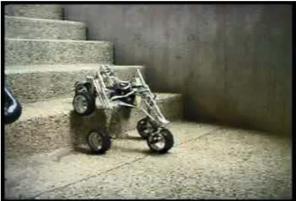
Shrimp : EPFL, 2008 (Link-mechanisms)
