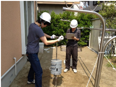
Swedish weight sounding test in Urayasu Kiyota Laboratory, Institute of Industrial Science, University of Tokyo
