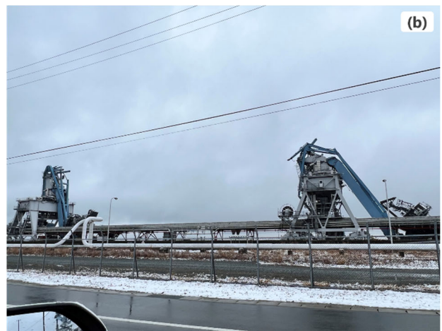
Fig.9 (a) a 130m-long crack on the carriageway in Quay No. 5, (b) Coal unloading machine with ruptured transverse beam
