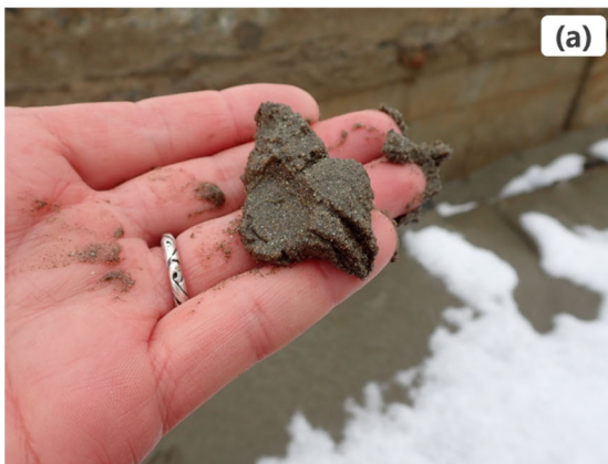
Fig.8 (a) Sand ejecta taken from a quay wall block, (b) Particle distribution curve and the diameter range of sand prone to liquefaction
