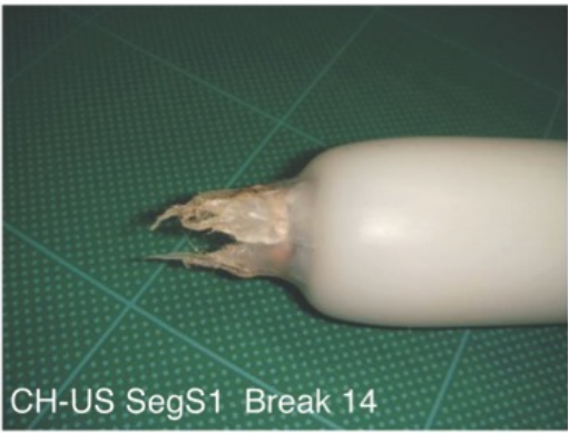
Fig. 2. Broken cables recovered during cable repair operations. Upper picture: break of an armoured type cable recovered during break 2 repair (located in Fig. 1). Lower picture: break of a lightweight type cable recovered during break 14 repair (located in Fig. 1).
